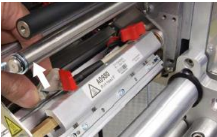
Fig.2. Removal of Printhead Cables
